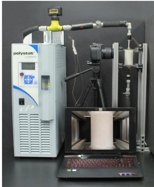
Fig. 1: Image of the experimental setup with the cylindrical TES system containing coconut oil.
