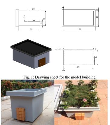
Fig. 2: The two model buildings used in the experiment (left without rooftop garden while right with rooftop garden).
