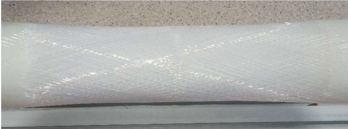
Fig. 1: Cross-wound hollow fibres inside the PHFHE.
