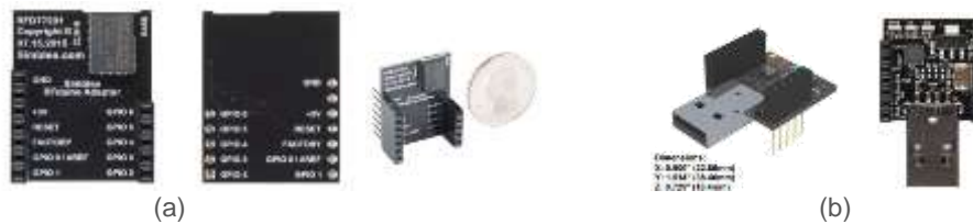
Fig. 9: (a) RFDuino - Simblee DIP (RFD77201 Simblee 7-pin DIP); (b) RFD22121 USB Programming Shield.
