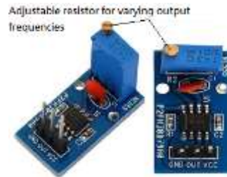
Fig. 7: The square wave signal generator NE555 with Frequency adjustable.
