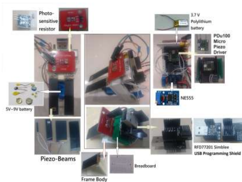
Fig. 16: Micro piezoelectric robot integrated with Rduino-Simblee, PDU100 Micro Piezo Driver and Photosensitive resistor
