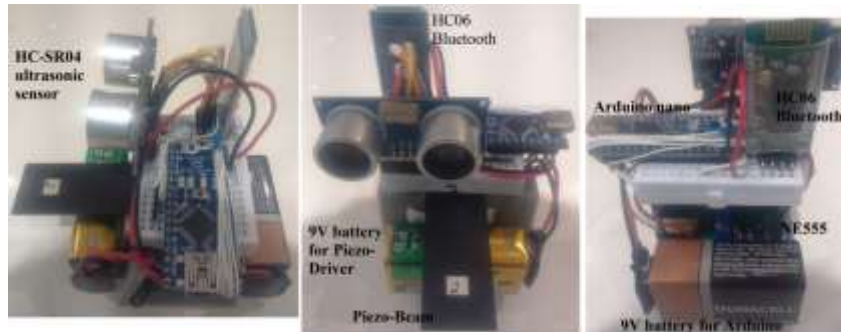
Fig. 14: Micro piezoelectric robot integrated with Arduino nano, self-made miniaturized Piezo-driver, HC06 Bluetooth and HC-SR04 ultrasonic sensor.
