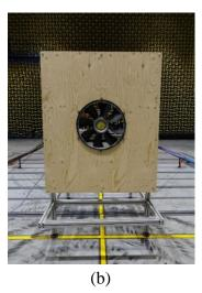
Figure 1: (a) - Scheme of the semi-anechoic chamber with microphones positions, (b) - Picture of the Fan test stand
