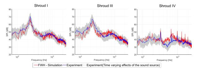
Figure 5: Validation of the sound pressure level spectrum calculated with the FWH acoustic analogy by the measured data for Shroud I, Shroud III, Shroud IV variant
