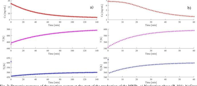
Fig. 2: Dynamic response of the reaction system at the start of the production of the MNPs. a) Nucleation phase (R-101), b) Growth phase (R-102).
