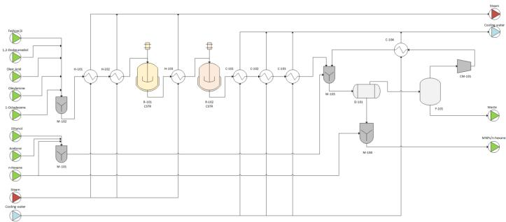
Fig. 1: Diagram of the MNPs production process by thermal decomposition.
