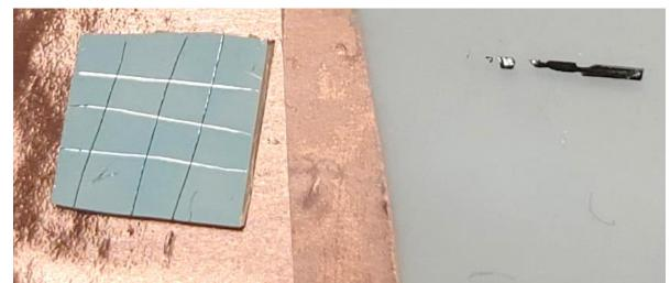
Fig. 8: Peeling test of the nano-twinned (111) Ag film with a thickness of 9 µm on a 0.1 µm Ti-coated (111) Si substrate.
