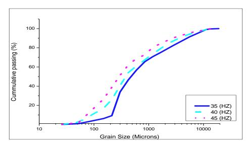
Figure 1: Particle Size Distribution of the VSI product at different rotor speed
