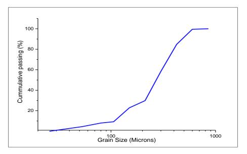
Figure 2: Particle Size Distribution of the Middle Group Ball mill product
