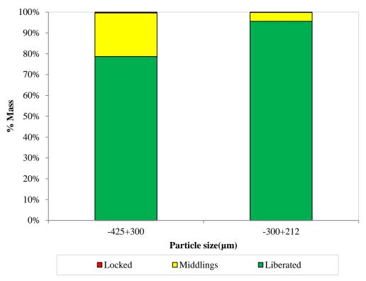
Figure 5: Degree of MG Chromite liberation analysis
