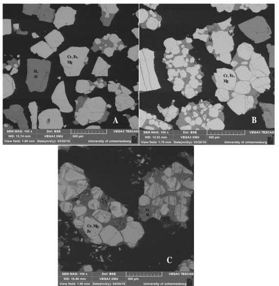
Figure 4: Surface morphology of the MG crushed product
