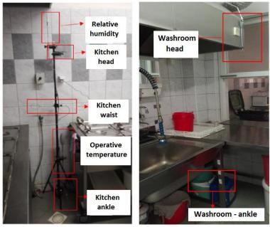
Fig. 2: The location of the probes in the kitchen and washroom
