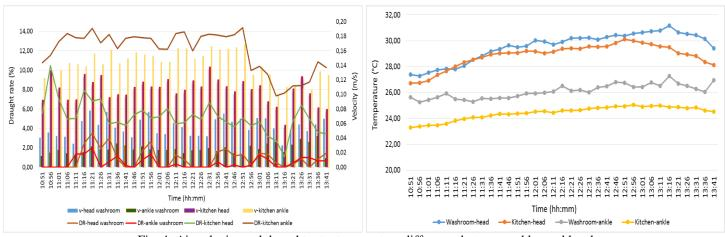
Fig. 4: Air velocity and draught rate, temperature difference between ankles and head
