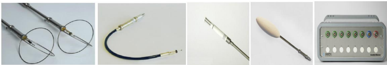
Fig. 1: Measurement probes of temperature, velocity, humidity, operative temperature and main frame.
