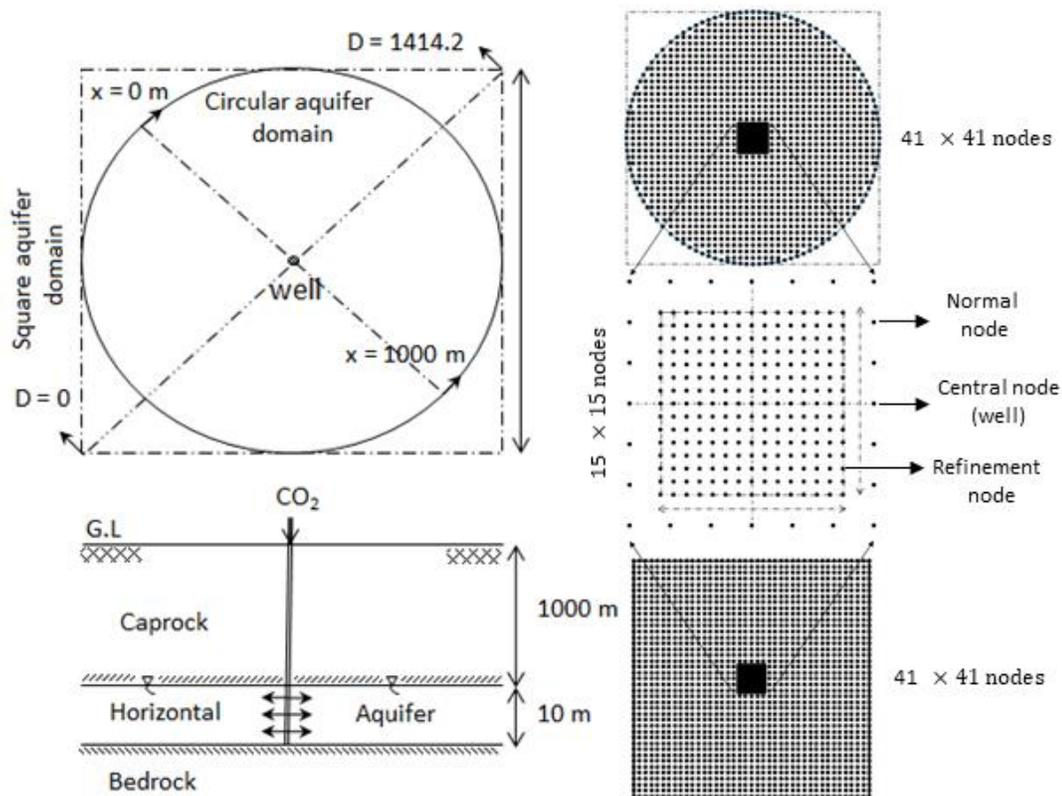
Fig. 3: Set-up of the square and circular shaped horizontal adapted from Ladubec et al. [3] with its EFG nodal discretization.
