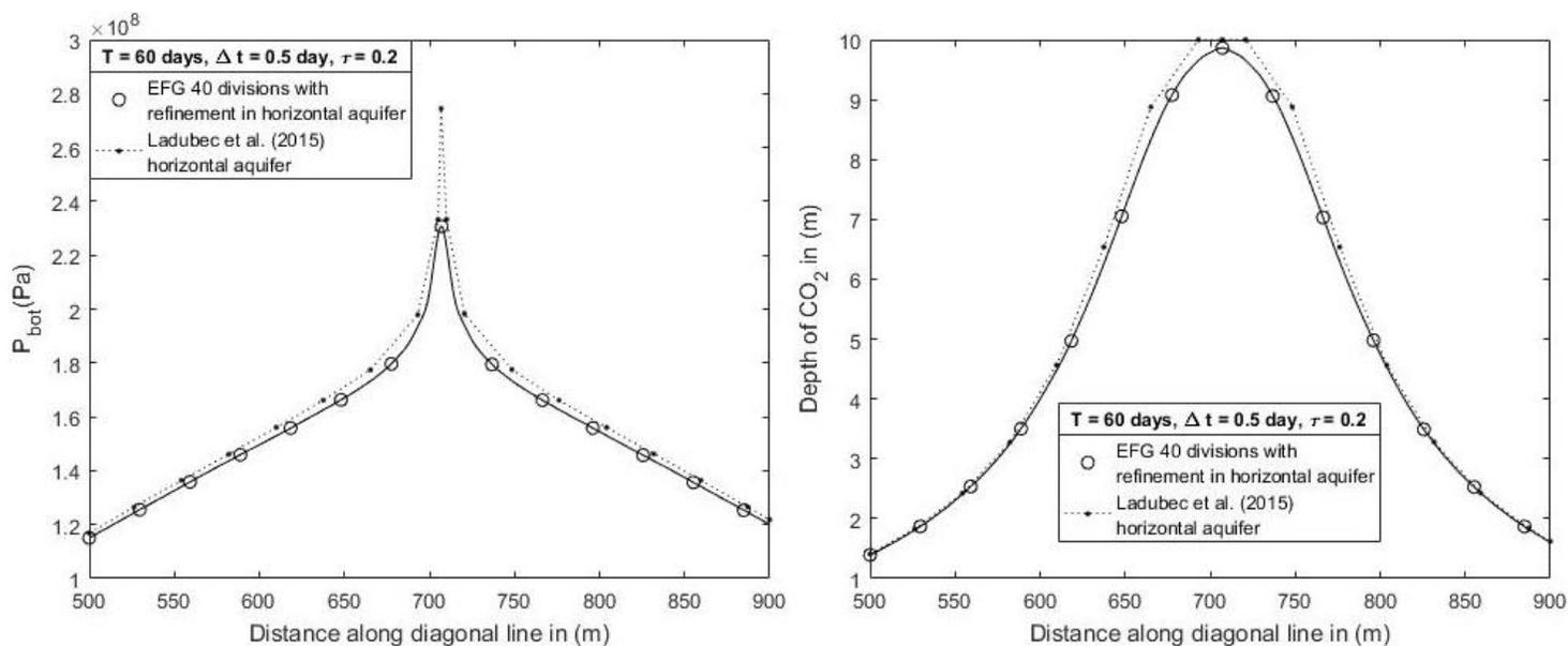
Fig. 6: Comparison of numerical XFEM and EFG model for pressure and average CO<sub>2</sub> saturation from square aquifer domain.
