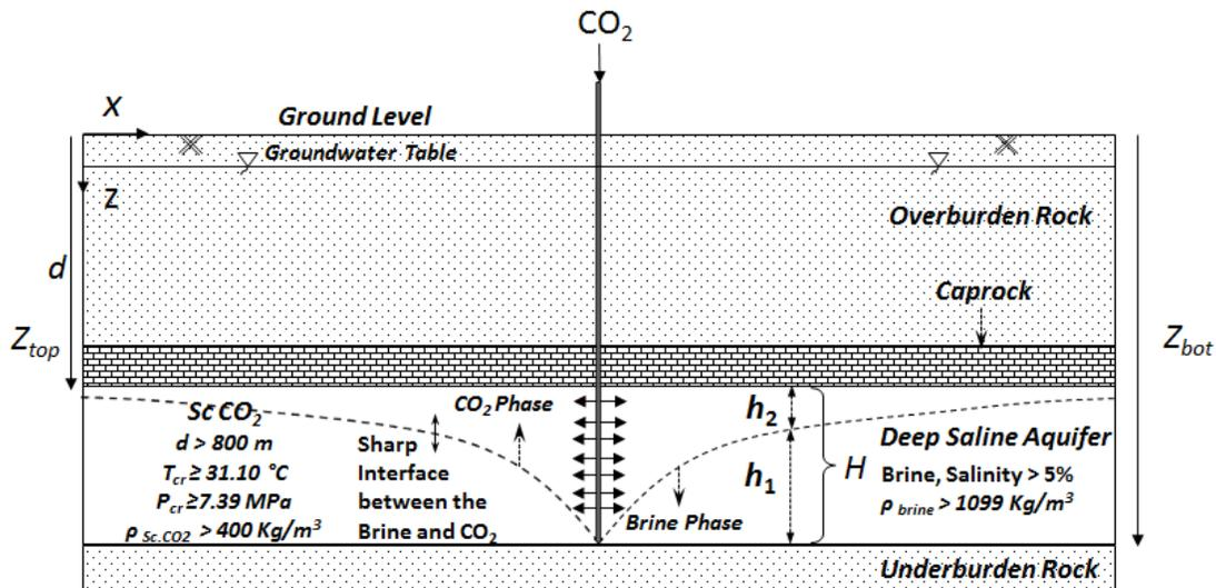
Fig. 1: A conceptual diagram of CO<sub>2</sub> sequestration model with defining parameters.
