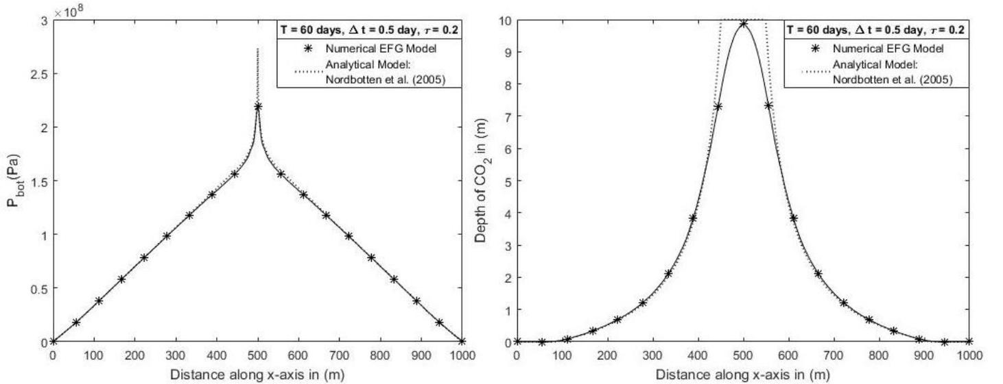
Fig. 5: Comparison of analytical and numerical EFG model for pressure and average CO<sub>2</sub> saturation from circular aquifer domain.
