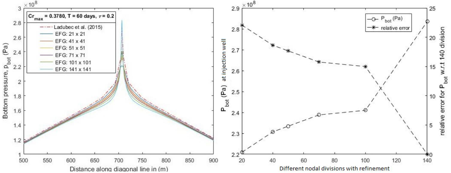
Fig. 4: The pressure solution and its EFG nodal independent analysis at maximum courant number of 0.3780 and  $\tau$  is 0.2.
