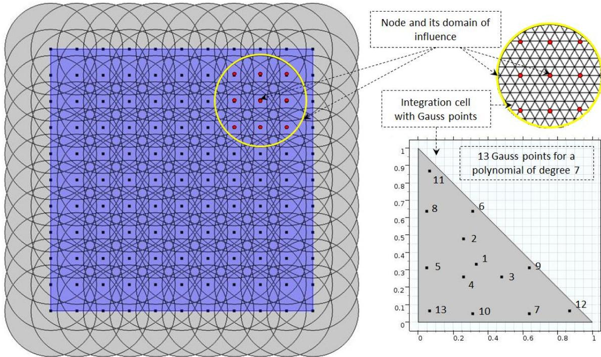
Fig. 2: The domain of influence (DMI) for the field nodes with background integration cells and Gauss points.
